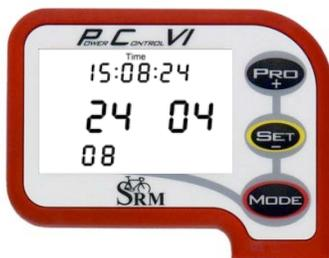
Hold **SET** for about 3 seconds to enter the Setup mode.
