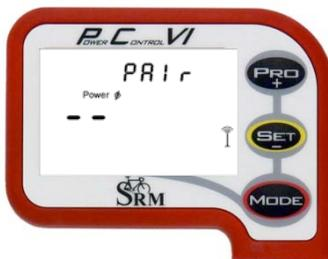
The Antenna symbol
