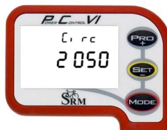
The third screen shows the setup menu for the wheel circumference in Millimeter [mm].
