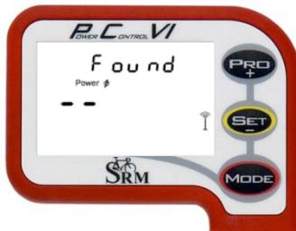
When a sensor is found, the PC VI will show "Found" in the top line, alternating with the sensor's serial number.
