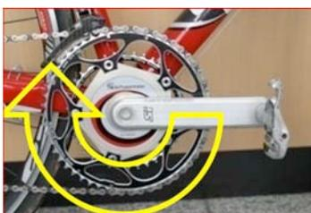
If the top number is zero, turn the PowerMeter on by pedaling forward. Then, **let go of the crank and make sure nothing is touching it.**
