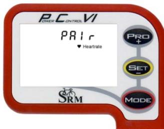
To pair another sensor, press **MODE** once quickly to get back to the device selection Menu. Continue with pairing the heart rate sensor and speed sensor.
