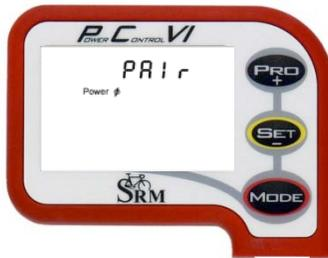
Hold **PRO+** for about 3 seconds to enter Sensor Pairing mode.
