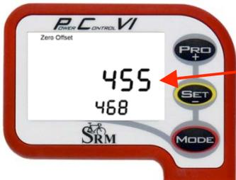
After the top number stabilizes, press **SET** to store the new **Zero Offset** of the PowerMeter.
